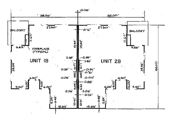
NOTE: ALL WALLS 0.35' THICK UNLESS NOTED. EXTERIOR FREPLACE WALLS 0.29' THICK.
